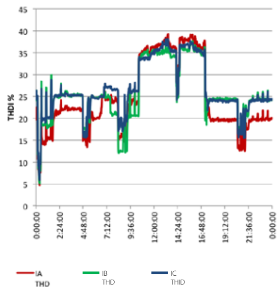
Figure 9: Harmonic Current distortion
